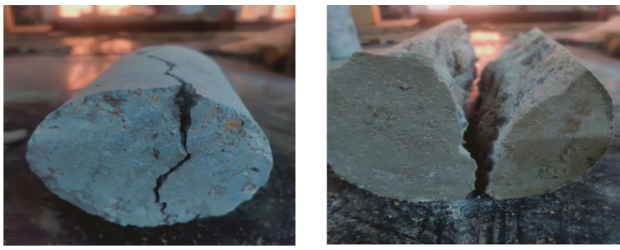
Fig. 4 Cylindrical tested specimens for split tensile strength
